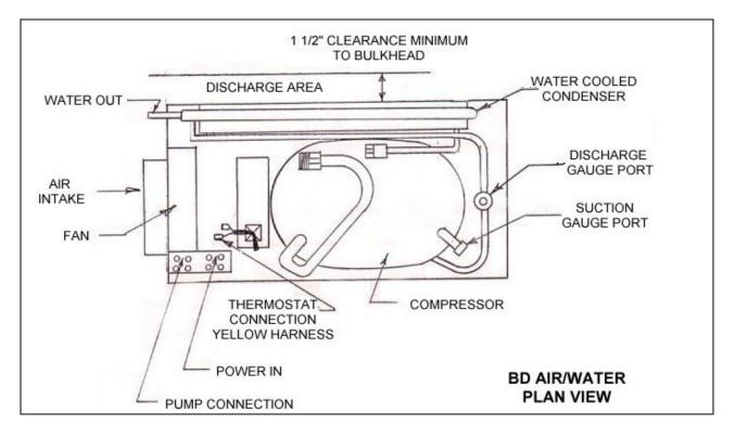
Service access and installation requires that the front, left end (inlet) and back (condenser) air outlet be exposed. A duct hose will require 4 inches of clearance past the end of the cabinet.
